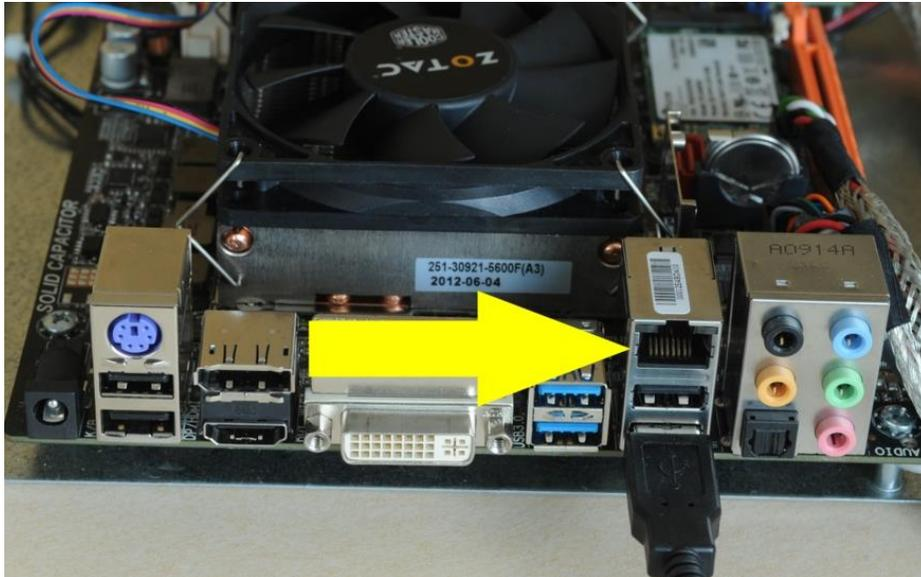
Figure 2: The other end of each blue Ethernet/network cable seen in Figure 1 should be plugged into the Ethernet/networking ports designated by the yellow arrow on the gaming motherboard in Figure 2.
