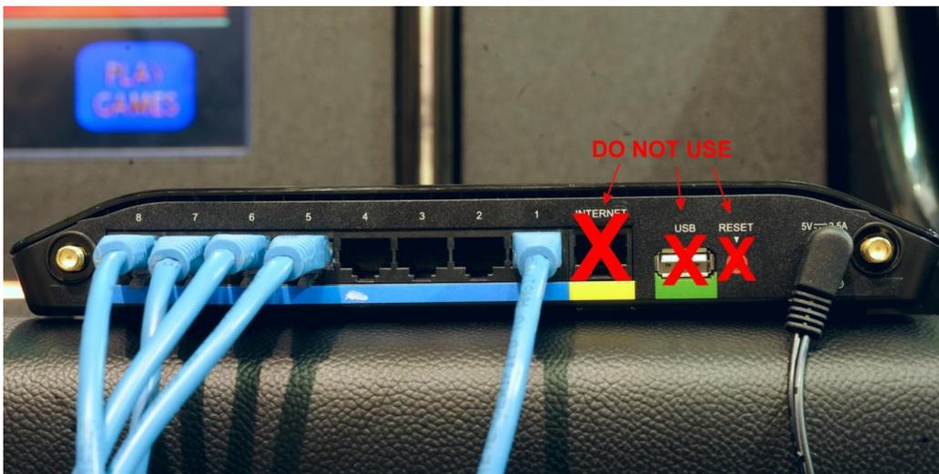
Figure 1: Power cord (black) and Ethernet/networking cables (blue) plugged into the back of an 8-port router.
